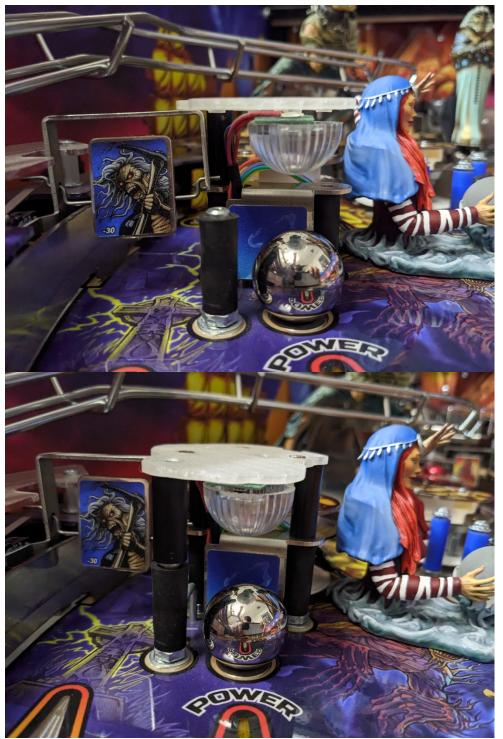
6. With the mounting bracket now in place, can take the model and pop into place. To help the wiring maintain a flush placement, each wire should exit the rear in the same order. Arrange the color wires as they exit the back if needed. Don't worry if theres too much slack of the wiring. Will be adjusted on the final step.
