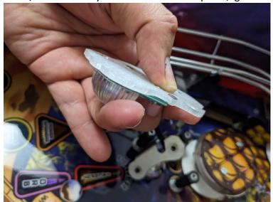
4. Set the Clairvoyant model to the side of its install location and run the cable through the opening on the metal plate that was behind the target ball, and run the connector down hole where the current dome light is.
