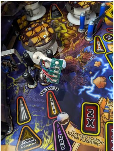
3. New Mount – Use the included small screw for the downward light. While holding screw in place, place the LED board and the dome cover in its original configuration that was in the stock mount. Tighten the screw/nut. NOTE: If your dome line had a spacer, ignore it as I built in one to the mount.
